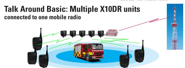
The XIB-TA allows users in a vehicle with multiple X10DRs connected to the mobile radio to have local (talkaround) operation where by those users can talk locally "off net" by using the orange side button as a secondary PTT. To talk over the radio channel, the normal PTT button is used. All host radio receive traffic will be heard regardless of local talkaround PTT status.
