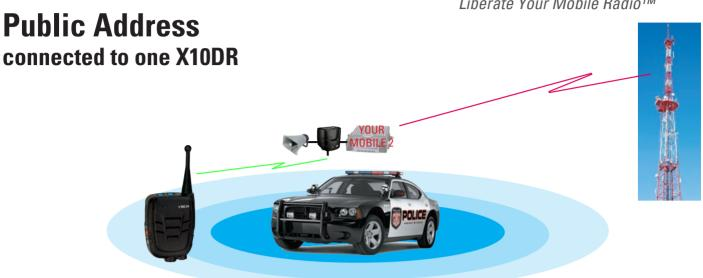
The XFB-MR can also be used to allow the XFB-MR second port to be attached to the vehicle's Public Address system to allow the user to talk over the vehicle's public address system by pressing the X10DR microphone's orange button.
