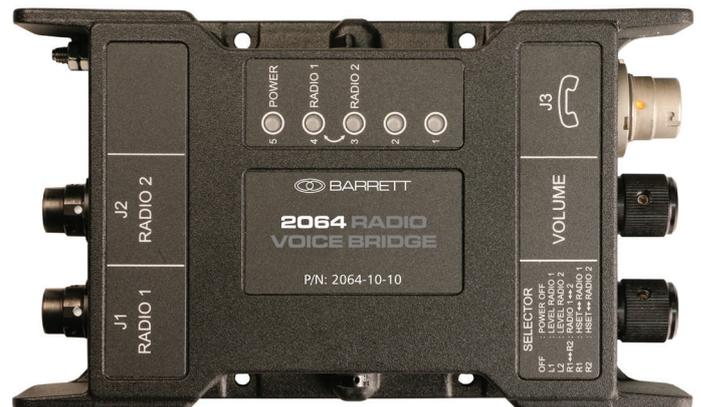
Cross-connecting the audio between network 1 and network 2 forms a bridge between the radio networks over which the 2064 user can both monitor and communicate. The voice bridge is automatically activated whenever voice is detected on either network.
