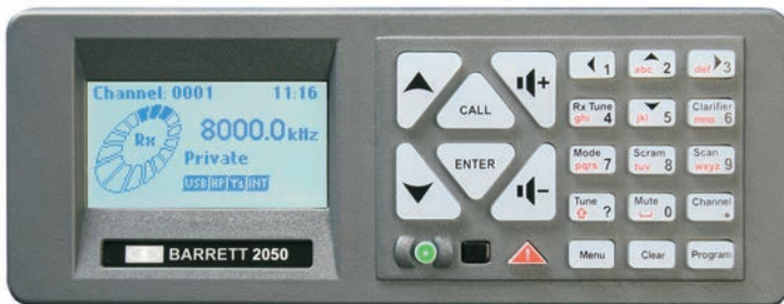
Barrett 2050 HF transceiver front panel
