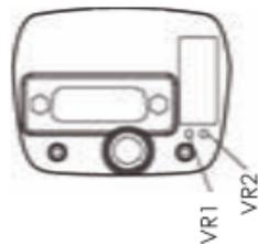
\* Mic audio can be increased to >400mV via VR1 trim pot - use hole in base of mobile charger.
