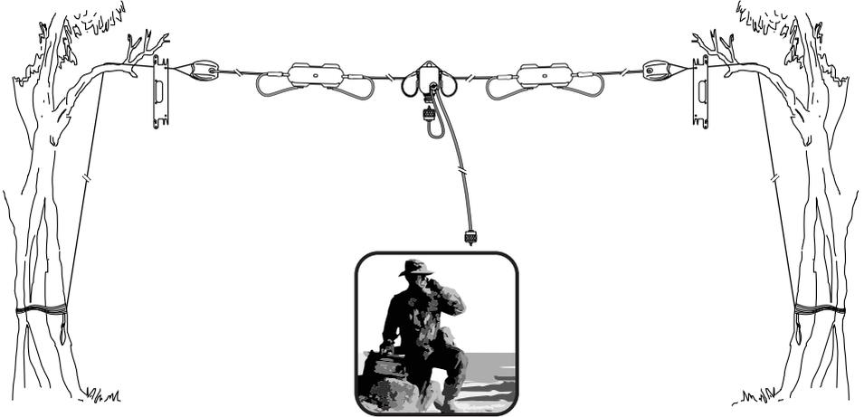
**Inverted V Configuration** The inverted-V configuration has a more omni-directional pattern than the horizontal configuration, with lower maximum gain. The ends of the antenna should be at least 0.5m above ground. Suitable mainly for NVIS and medium distance communication.
