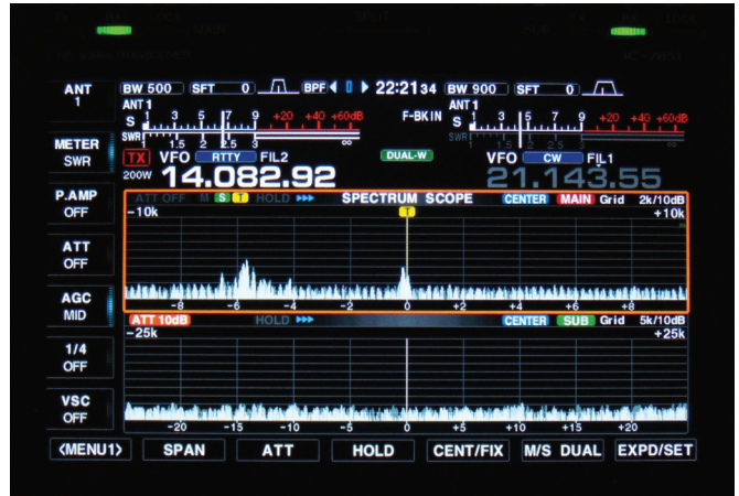
Figure 3 — A view of the front panel display of the IC-7851 as in Figure 2, except we now have elected to show spectrum displays of both receivers and the meters are in a more compact format. Note that one receiver is set up for RTTY, one for CW, and the spectrum displays are set for different display widths — there's a lot of flexibility here. The spectrum displays can show panadapter views, as shown, or waterfall-type displays, or both. They can be set to show a fixed portion of the band, useful for monitoring, or can be centered around the tuned frequency.
