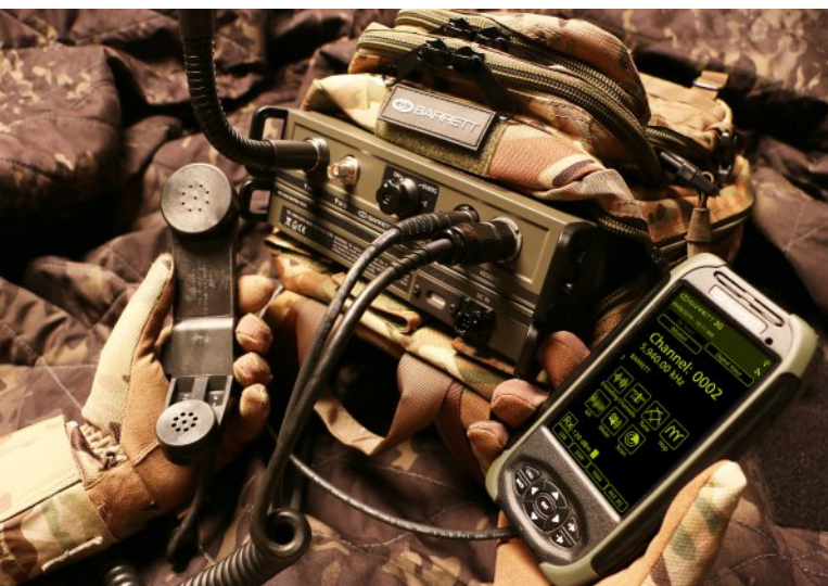
Barrett PRC-4090 HF SDR manpack with multicam daypack and optional H250 handset. Remote cable up to 50m.
