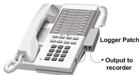
Figure 35: Digital Desk Phone with Logger Patch
