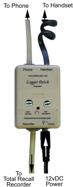
Figure 36: Logger Patch Wiring - Standard Headset
