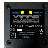
XPB-C14B In-line bank charger enables charging on vehicles with after-hours isolated vehicle batteries
