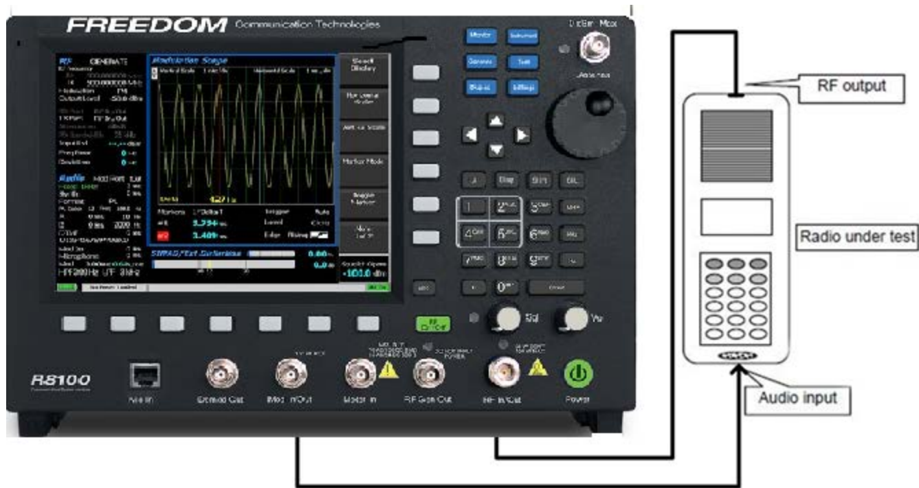
Figure 5.1.1-1 Setup for FM Transmitter testing
