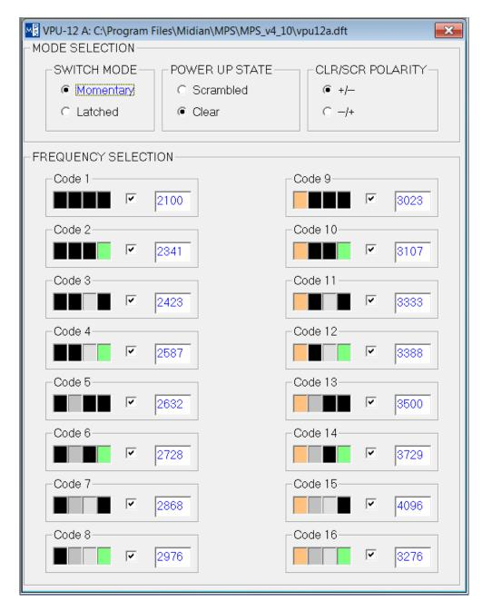
Switch Mode: Select whether the switch being used for mode selection is a momentary or latched switch.
