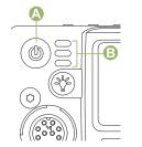
After a short time, the red, yellow and green LEDs B light up. The display then shows Zone and channel text, and menu items display on the screen.
