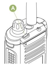
The Top Lightbar (A) indicates the secondary function of MFK and also the status of Intelligent Lighting.
