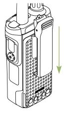
2 To remove the clip, use a flatbladed object to press the belt clip tab (A) away from the radio. Then, slide the clip upward and away from the radio.
