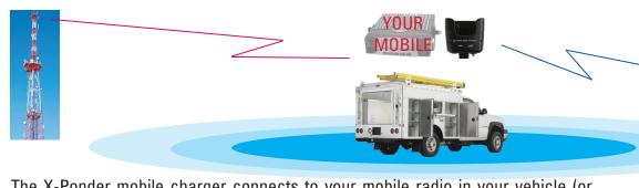
The X-Ponder mobile charger connects to your mobile radio in your vehicle (or office control station) It passes all voice traffic to and from the secure wireless microphone.
