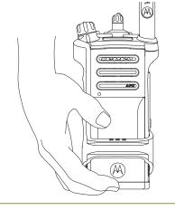
4 Push at the bottom of the radio until the radio is released from it.
