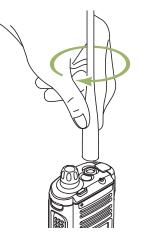
**3** To remove the antenna, turn the antenna counterclockwise.
