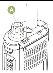
The Top Lightbar (A) indicates the secondary function of MFK and also the status of Intelligent Lighting.
