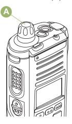
To increase the volume, rotate the On/Off/Volume Control Knob (A) clockwise.
