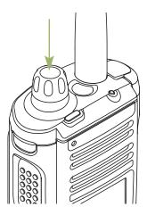
Rotate the **On/Off/Volume Control Knob** clockwise until you hear a click.
