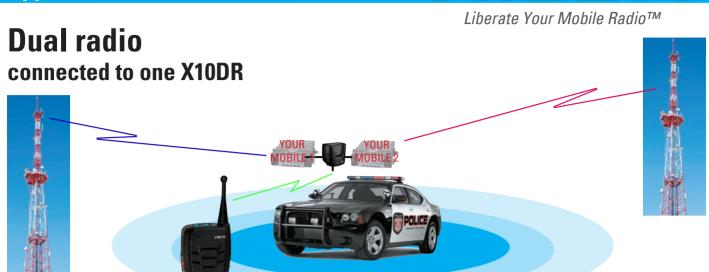
The XFB-MR can be used to allow 2 mobile radios to be connected to the one X10DR unit. A unique marker tone\* is attached to the tail of each secondary radio reception to inform the user which radio's audio they have just heard. The XFB-MR unit can be configured by way of a dip switch to either A/ maintain the secure microphone's emergency functionality on its orange button, or to B/ use that button as a PTT to transmit on the secondary radio's channel.
