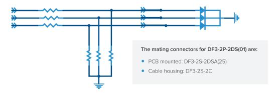
A DC power interface is provided through a 2-pin Hirose DF3-2P-2DS(01) connector with the following pinout:
