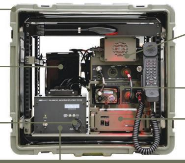
Radio quipment quickly removable. RFDS unit can be supplied without radio equipment so Barrett customers can use their existing equipment
