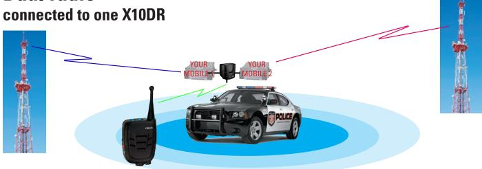
The XFB-MR can be used to allow 2 mobile radios to be connected to the one X10DR unit. A unique marker tone\* is attached to the tail of each secondary radio reception to inform the user which radio's audio they have just heard. The XFB-MR unit can be configured by way of a dip switch to either A/ maintain the secure microphone's emergency functionality on its orange button, or to B/ use that button as a PTT to transmit on the secondary radio's channel.
