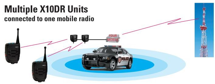
The XIB interface box allows multiple X10DR's to be connected to the one mobile radio. All units can hear each others communications as well as the conversations over the network. The interface unit connects to the host radio via the XMC series interface cable.
