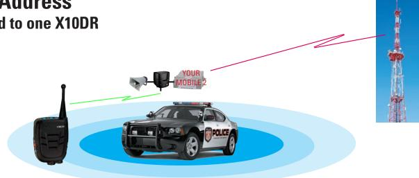
The XFB-MR can also be used to allow the XFB-MR second port to be attached to the vehicle's Public Address system to allow the user to talk over the vehicle's public address system by pressing the X10DR microphone's orange button.
