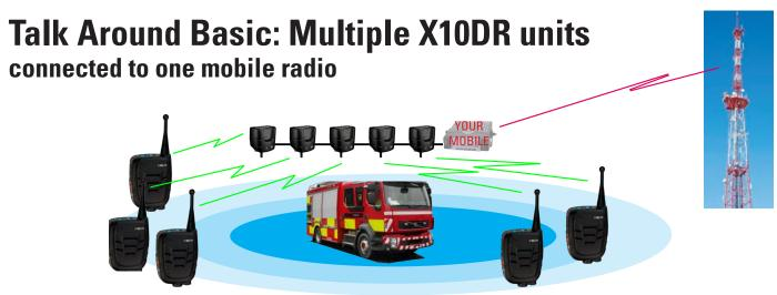
The XIB-TA allows users in a vehicle with multiple X10DRs connected to the mobile radio to have local (talkaround) operation where by those users can talk locally "off net" by using the orange side button as a secondary PTT. To talk over the radio channel, the normal PTT button is used. All host radio receive traffic will be heard regardless of local talkaround PTT status. **Note**: No remote triggering of the host mobile radio's emergency function is possible in this configuration
