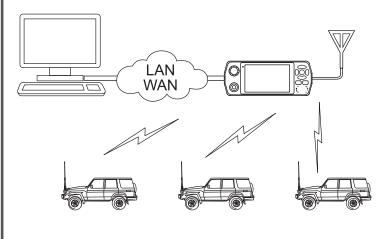
This scenario has 3 mobile transceivers, each with 6 channels programmed - 4 for voice transmission and 2 exclusively for consecutive GPS Push transmissions.
